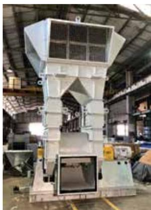
DIDW API 560 FD Fan with a common inlet filter/silencer, special coating and disjointed base for a refinery application.
