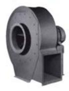
FLANGED INLET & OUTLET- Pre-punched flanged inlet and outlet simplify duct connection. Inlet flange is a formed steel ring bolted to the inlet. Outlet flange is flat bar welded to housing discharge.
