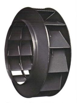
Rugged, Class III Wheels Class III wheels have reinforced blades plus heavy shafts and bearings to extend the rated duty to 15" static pressure. Sizes 20 to 44-1/2.
