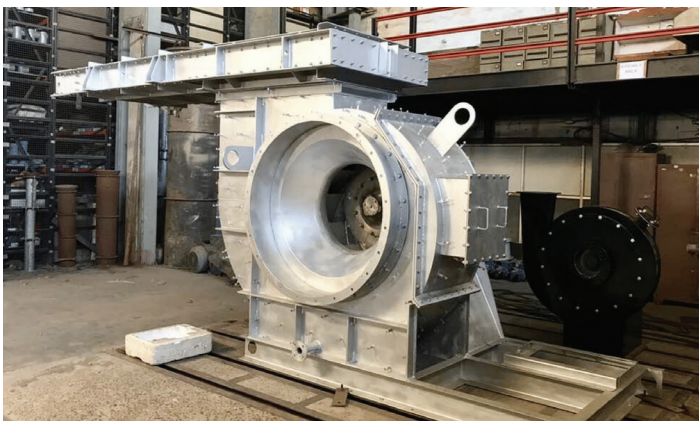
Design 6105 Size 4412 Arrangement 9H 80% Width ID Fan used for hot air recirculation at a speciality fluorochemicals plant in India.
