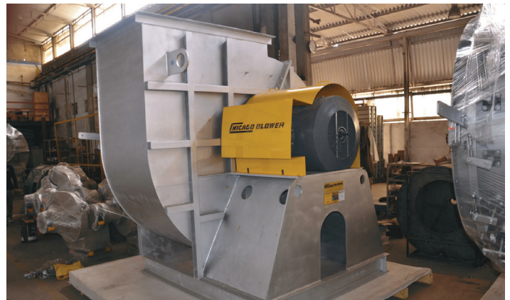
This Design 1911 AF Wheel Size 4900 Arrangement 4 with IVD, AMCA Spark Resistant Construction "Type C" & Variable frequency drives is for the ventilation of a Gas Turbine compartment.
