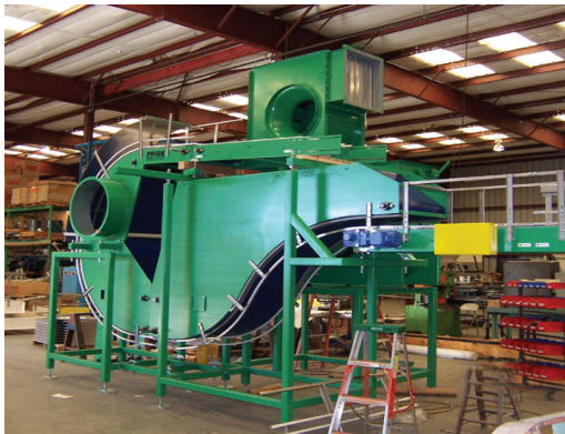
SQAD Direct Drive Fan used in a conveying system application.
