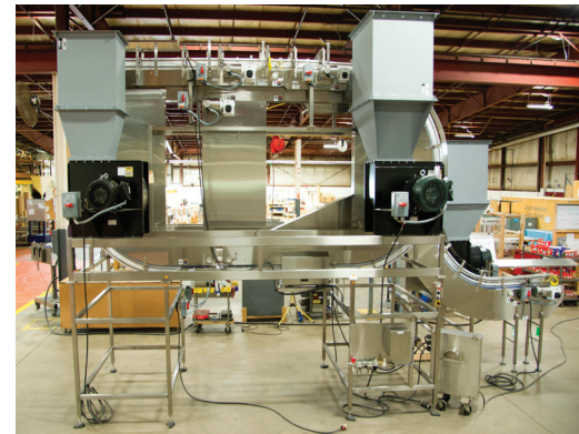
Two SQAD Fans being used in a conveyor vacuum rinser application.
